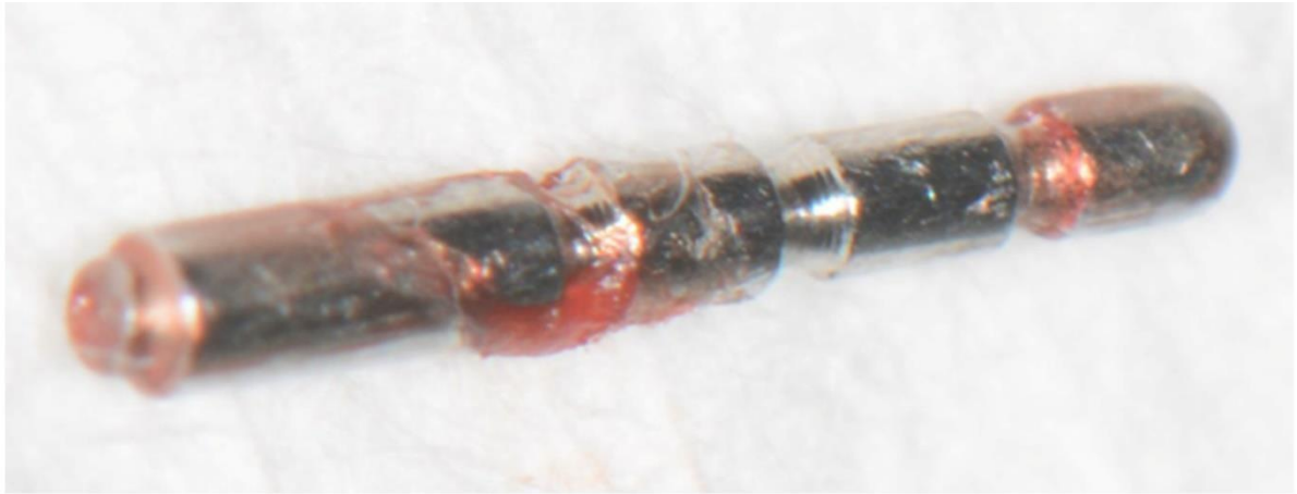
Fig. : The surgically removed fragment tip of a periodontal probe type AE P OWP.
